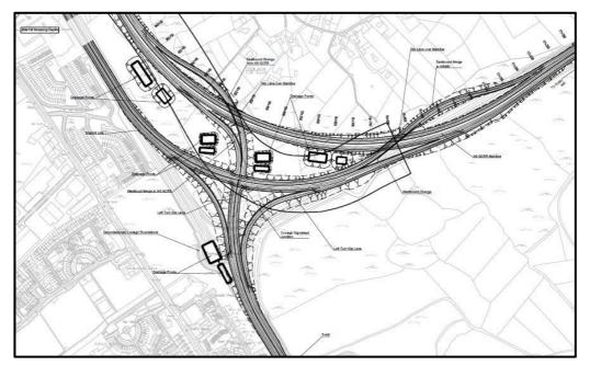
This junction layout addresses the issues raised above by including an at-grade signalised junction on the existing network connection, retaining priority on the N6 GCRR, retaining design speed on the N6 GCRR at 100km/h and also results in removal of some structures and a reduction in construction complexity.
