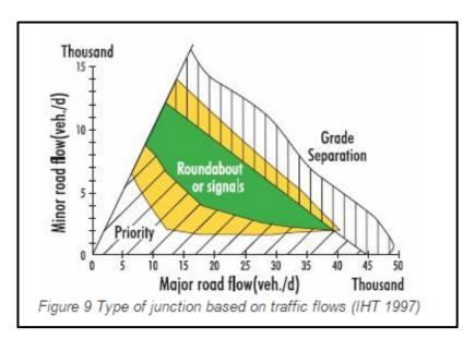
Phase 2 traffic analysis showed that the junctions contributed to significant delay along the key routes which were assessed to establish the performance of options. Therefore, a solution that offers a resolution to these significant delays has the benefit of contributing significantly in the economic assessment of benefits. As congestion relief is a key objective of the proposed scheme, grade separation is the preferable junction form on the dual carriageway section.
