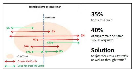
*Note:* arrows include traffic in both directions, inclusive of trips both into the zone and out of the zone
